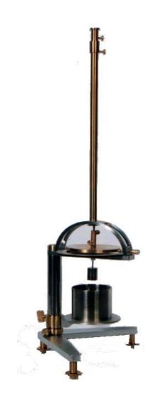
Developed with the Ceramic Industry in mind, (but easily modified for other use), the "Payne" Torsion Wire Viscometer is simple to use and maintain.
